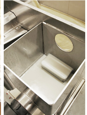
Clean coolant returned to sump
